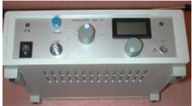
Figure 8.9: Electrical stimulator TMG – S1 was used for generating electrical stimulation in protocols A and B and experiments on toad isolated gastrocnemius.
