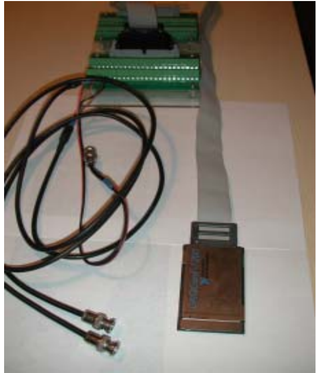
Figure 8.6: Input-output interface for transferring collected data together with the connection-board (connecting BNC cables from measuring instruments).
