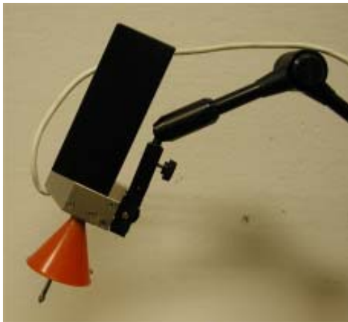
Figure 3.5: Displacement sensor with the spacer.
