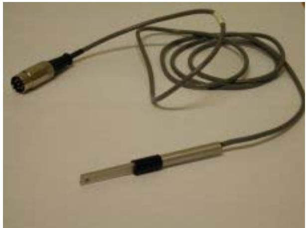
Figure 8.3: Force sensor for measuring longitudinal responses of toad gastrocnemius
