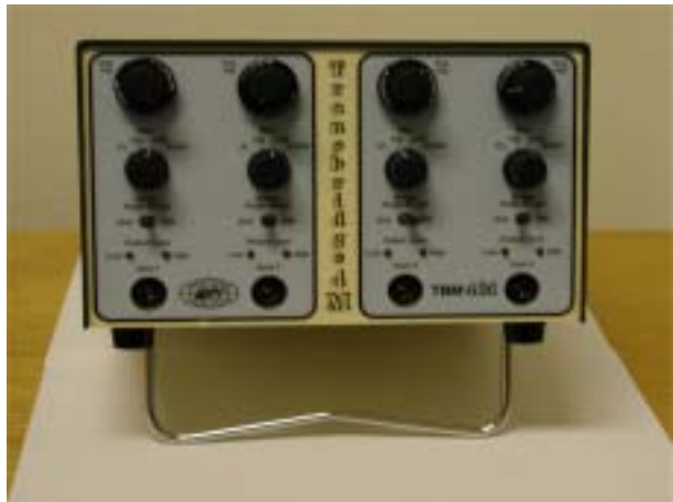
Figure 8.5: Differential amplifier TBM4M.
