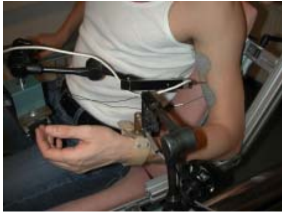
Figure 3.3: Force sensor, displacement sensor and stimulation electrodes position for measurement on m. BB at elbow angle of 1.75 rad.
