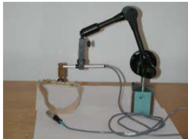
Figure 8.2: Force sensor for measuring longitudinal responses of human skeletal muscles
