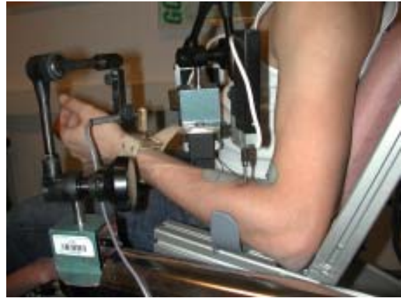
Figure 3.4: Force sensor, displacement sensor and stimulation electrodes position for measurement on m. BR at elbow angle of 1.75 rad.
