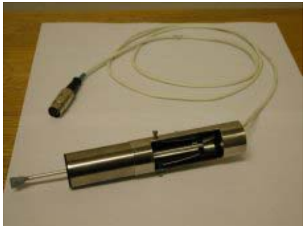
Figure 8.4: Displacement sensor for measuring transverse responses of toad muscle belly
